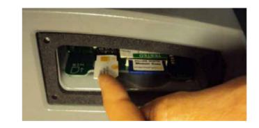
When the sim card is in its place, fasten the cover plate for the SD card back in its place using the four pozidrive
